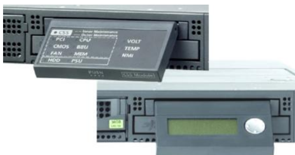
Fig. 14: Local Service Panel (LSP; above) and Local Service Display (LSD; below)
